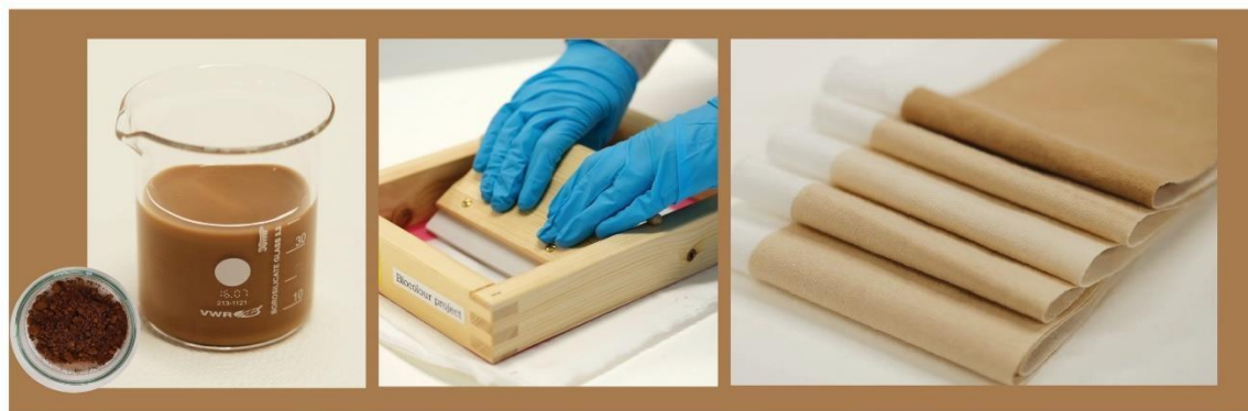
Figure 1. Paste prepared using Kraft lignin as colorant (left) and cotton fabric screen-printed with lignin containing pastes (right).
