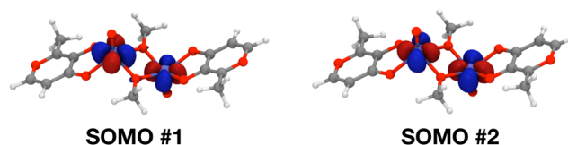
FIG. 12. A challenging case of strong and weak correlation: the [(\mu\text{OCH}_3)\text{VO}(\text{ma})]_2 dimer complex and its two singly occupied MOs. The three-body iFCI yields a singlet–triplet gap within 30 \text{ cm}^{-1} of experiment. 317
