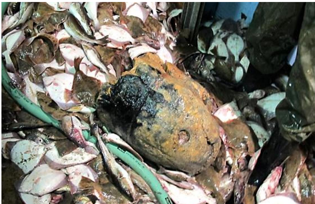
Figure 3. A lump of solidified sulfur mustard trawled up with fishes. As it contained explosives, it was emergency-relocated. 24
