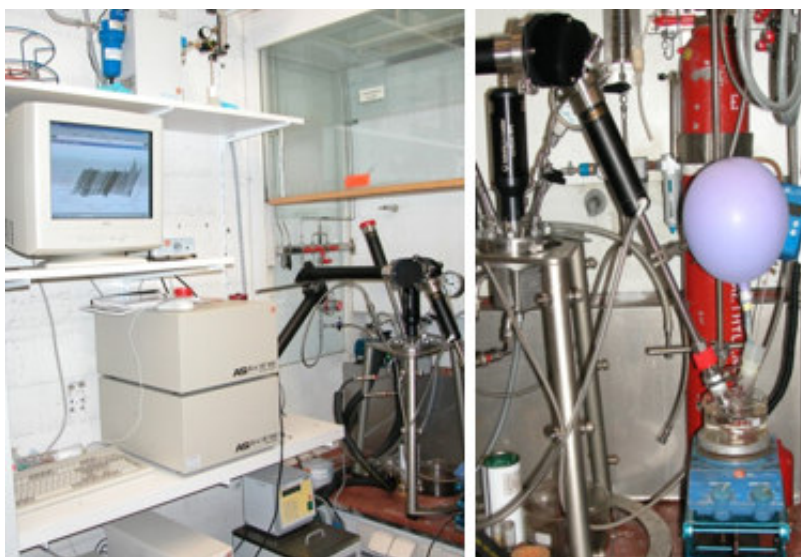
Figure 22. The experimental set-up used for in situ ATR-IR spectroscopy.
