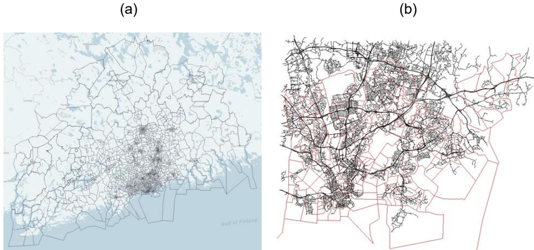
Figure 4. Traffic assignment zones: (a) for the extended area, (b) for the core area.
