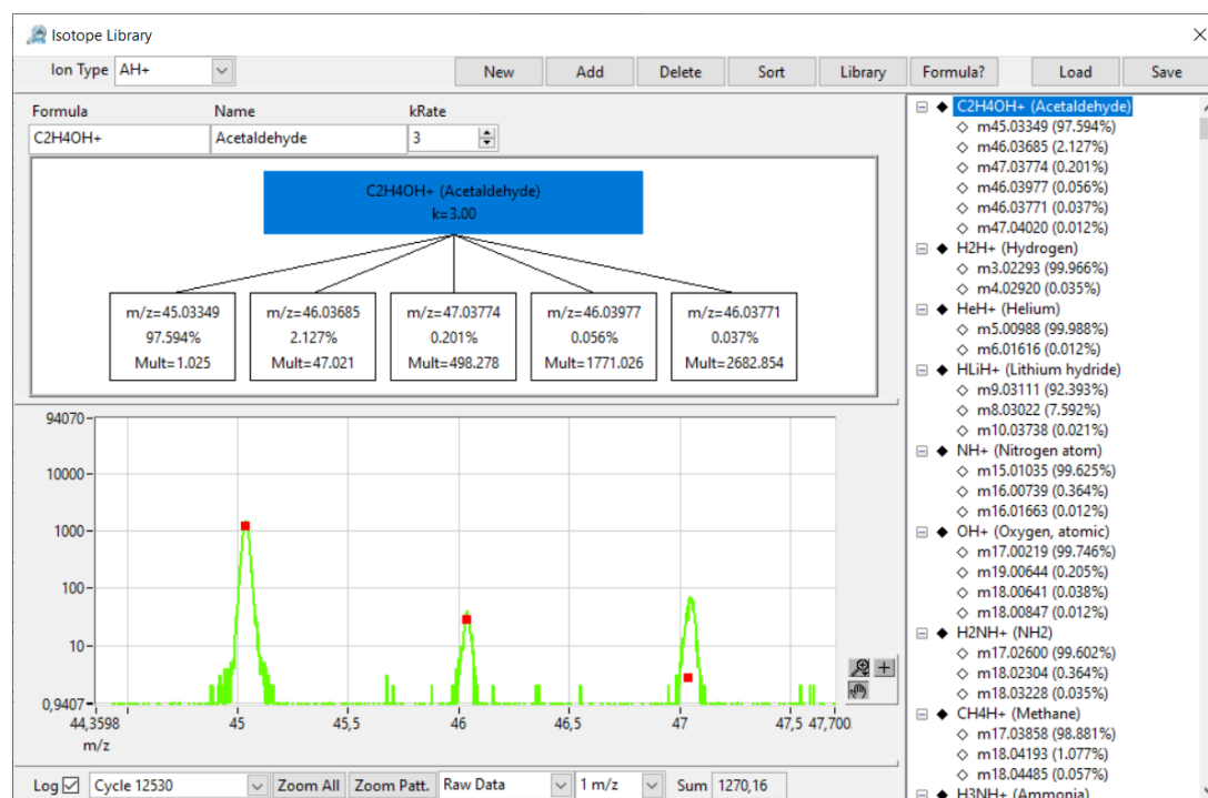
Figure 4.7: Screenshot of the Isotope Tool window. The theoretical isotope pattern is shown with expected m/z and abundances. The red dots represent the theoretical isotope pattern, and the green line represents the spectrum. For the third isotopologue, the theoretical pattern does not match the spectrum due to overlap with ethanol ( m/z 47).
