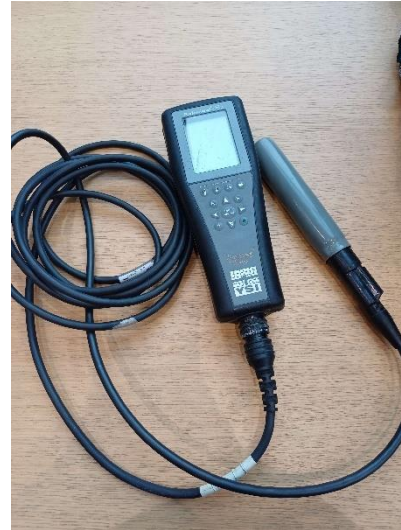
Figure 4. YSI device used to measure the physiochemical properties of water.
