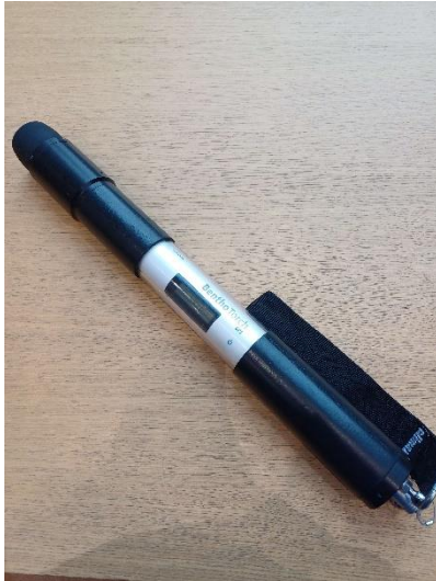
Figure 3. BenthosTorch device used for the benthic algal biomass measurements.
